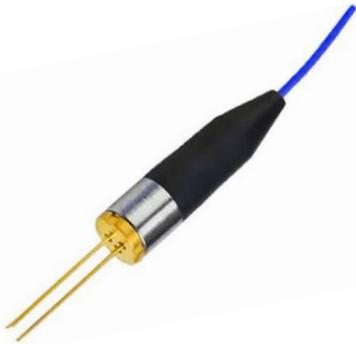
The PPF series fiber-coupled laser diodes are designed with a GaAs quantum well structure integrated with a grating configuration. These diodes feature a built-in photodiode for precise monitoring and feedback control of the laser's output power. Housed in standard TO packages, these diodes are pigtailed to a 1-meter long single-mode fiber terminated with an FC/APC connector. Each unit undergoes rigorous testing prior to shipment to ensure reliability.
